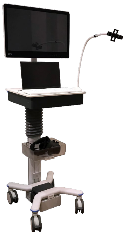
Figure 2. Endosight system overview: cart, medical display, laptop, and Oculus Rift-S paired with a Zed Mini camera.
